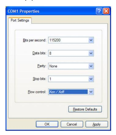
5. Switch on the power to the fusion box at the plug. The fusion should boot and speak to the PC. It should look something like below:
