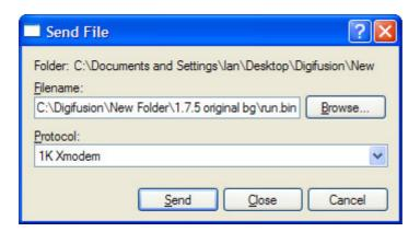
8. Click send then switch the power off and on at the wall socket for the fusion box. The file transfer window should appear.
