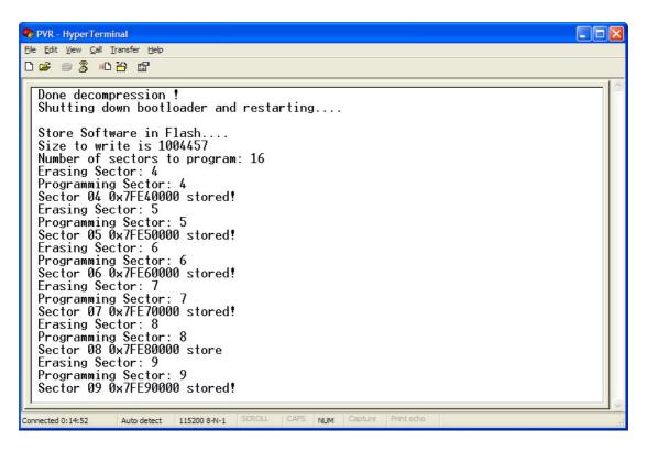
9. When the update is complete "Shutting down bootloader and restarting" will appear in the bottom of the hyperterminal window. The updating is over and Hyperterminal can then be closed down. The box should start up normally.
